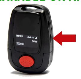
**Start the G-SAFE:**Press the bottom button for on the side 3 seconds or until you hear a 'beep' and feel a vibration
