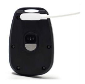
At the end of the shift, connect the device with USB magnetic cable to charger block provided for charging, so that it is full and ready for the next use. When battery reaches 100%, after a few minutes the device will shut off.
