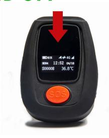
The screen will light up and display the percentage (%) of remaining battery, cell signal strength, and the current date. The G-SAFE is now ready for use. The screen will shut off after a few seconds, to display the screen, press once on the lower side button,.
